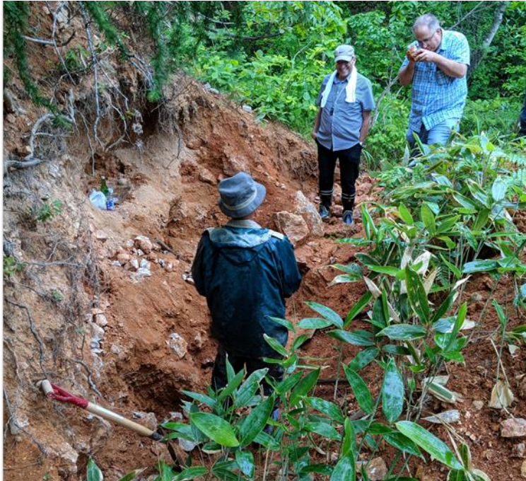
Pit excavated by local prospector, Mr. Masaru Nanjo, exposing the high grade ore veins (2 or more mineralized vein over a span of 6m)
