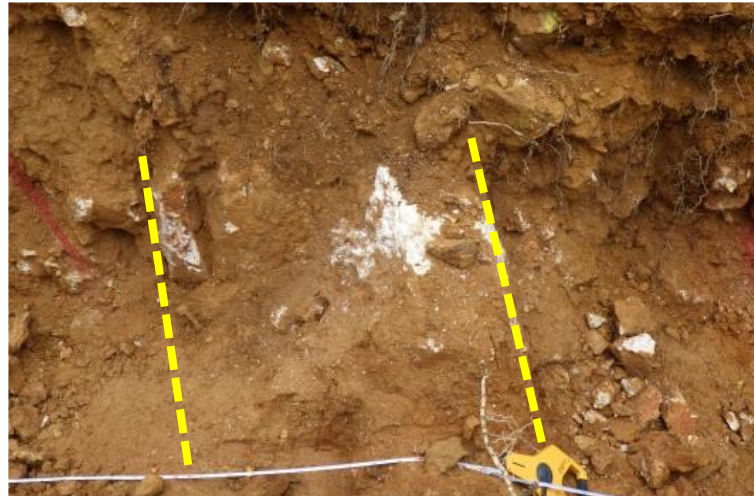
Milky white quartz vein at Trench 3 from 78.75-81.25m (~2.5m wide, N80°E 90°, up to 1.29ppm Au, 59.7ppm Ag)
