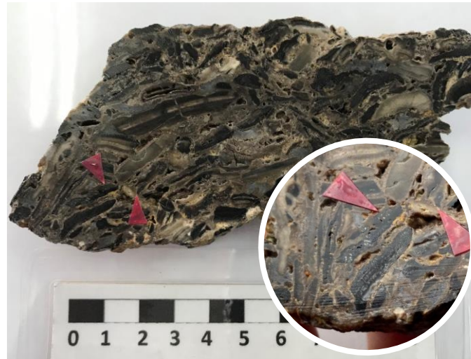
Honpi-style vein float, electrum and ginguero in the clast & matrix (16OM-012, 480ppm Au, 9660ppm Ag)
