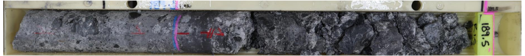
Clay matrix breccia in 200MS-001 from 189.00-189.5m (14.55ppm Au, 213 ppm Ag, 281ppm As, 196.5ppm Sb)
