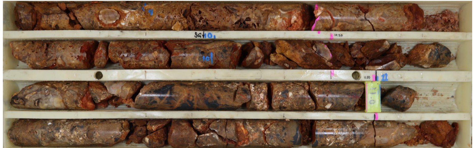
Honpi-style quartz vein in 190MI-009 from 9.35-10.2m (2.2ppm Au, 24.70ppm Ag), 10.2-11m (2.87ppm Au, 24.1ppm Ag), 11-11.95m (4.84ppm Au, 49.3ppm Ag)
