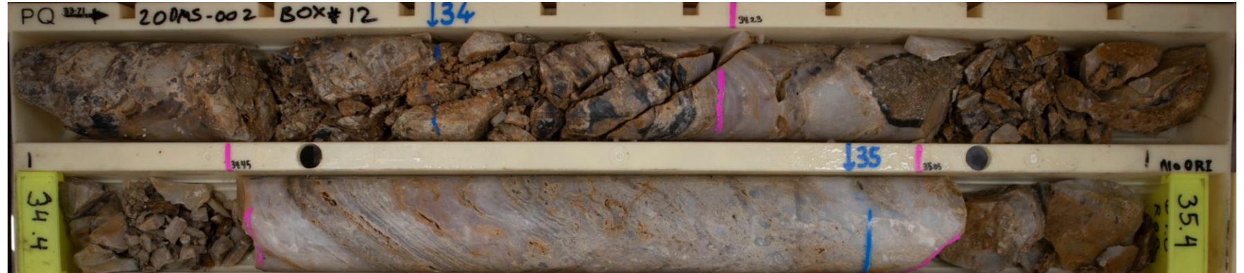
Finely laminated silica sinter in 20MS-002 from 34.23-34.45m (1.025ppm Au, 9.72ppm Ag, 236ppm Sb), from 34.45-35.05m (0.969ppm Au, 6.78ppm Ag, 345ppm Sb)
